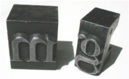
Type measurements were based the size of the metal block. Today it is a digital block.
